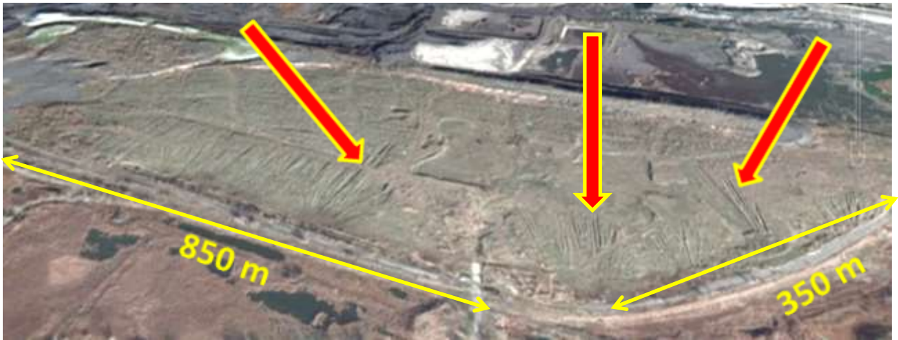
Figure A8.22: Upland drainage ditches and trays. Improper drainage of the tailings causes floor erosion of the talweg of a gully/ravine. The drainage system may be destroyed with further development of erosion
